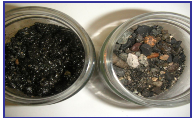
▲ Fig. 1-2: Ivey-sol® soil washing: pre and post treated soil from an industrial SER® soil washing process
